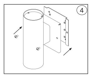
A. Align and attache faceplate to mounting bracket using the supplied 2 x 10-24 truss-head screws.
