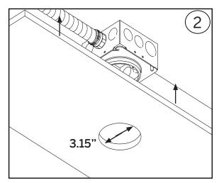
Install drywall or drop ceiling with a 3.15" diameter cutout.
