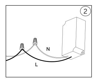
Connect line (black) and neutral (white) wires to corresponding incoming wires using wire nuts (supplied by others).
